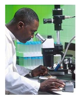
Figure 1.31: This scientist is using a stereo microscope, which is a light microscope with two ocular lenses (the microscope lense that is closest to the eye). The microscope is fitted with a digital imaging device that can take digital photos of what the researcher sees. (37)
