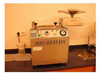
Figure 1.35: A worktop autoclave. Autoclaves commonly use steam heated to  $121^{\circ}C$  (250°F), at 103 kPa (15 psi) above atmospheric pressure. Solid surfaces are effectively sterilized when heated to this temperature. Liquids can also be sterilized by this process, though additional time is required to reach sterilizing temperature. (24)
