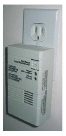
Figure 24.15: Home carbon monoxide detector (13)
