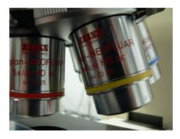
Figure 1.32: Objective lenses of a light microscope. (48)
