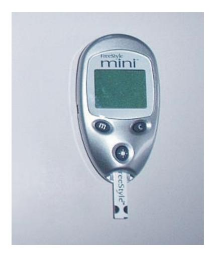
Figure 21.12: This is one type of meter used by people with diabetes to measure their blood sugar. Modern meters like this one need only a drop of blood and take less than a minute to use. (25)
