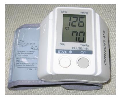
Figure 18.21: A digital sphygmomanometer is made of an inflatable cuff and a pressure meter to measure blood pressure. (22)
