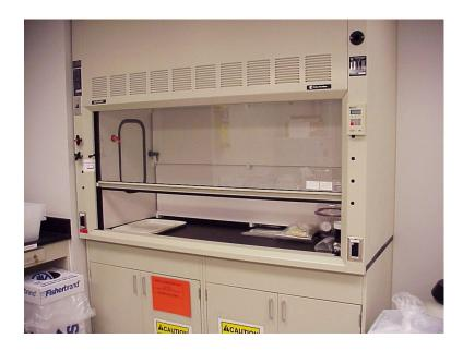
Figure 1.24: A laboratory fume hood. This laboratory hood sucks dangerous fumes out of a lab and allows researchers to work with dangerous chemicals without breathing them. (27)
