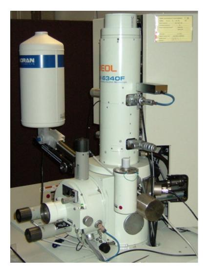
Figure 1.21: A scanning electron microscope. (6)
