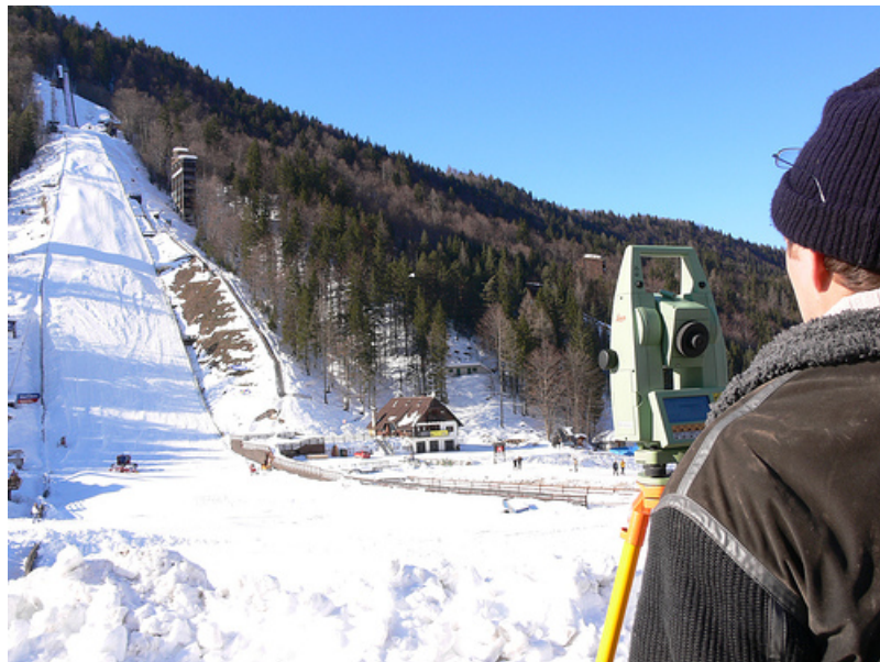
Figure 3: Using a laser to make a precise distance measurement.
