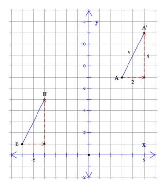
The arrow from A to A' is called a **vector**, because it has a *length* and a *direction*. The horizontal and vertical components of the vector are **2** and **4** respectively.
